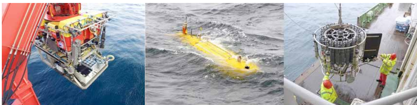
Figure 2. ISIS ROV; Autosub 6000; CTD rosette (Photo credits: NERC funded Deep Links Project - Plymouth University, Oxford University, JNCC, BGS)
